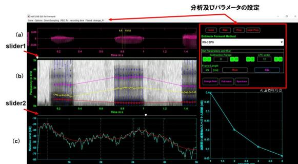
Fig.1 Formant Estimation GUI [1]
