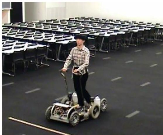
Fig. 1 Tread-Walk with wearable fNIRS
